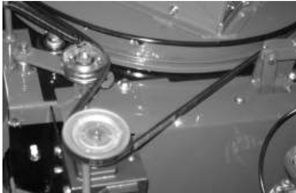
Figure 8 Hopper Belt Installation
