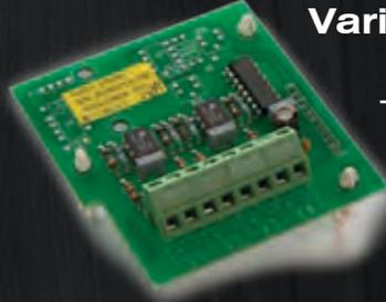
The Variable DC Expansion Kit is a small, auxiliary circuit board that allows you to connect equipment requiring a 0 to 10 V input, such as variable frequency drives or modulating valves.
