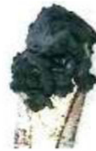
NLGI No.2 Multi-Purpose Polyurea caked, almost dry - FAILED after 1 season use
