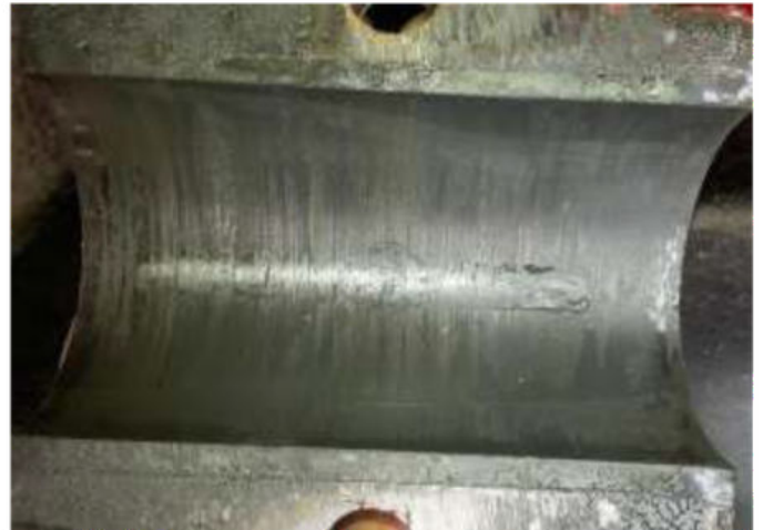
NLGI No.2 Multi-Purpose Polyurea caked, almost dry - FAILED after 1 season use
